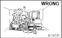
ventilation Have good when weldina or grinding painted parts. Wear dust mask when grinding
