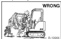
Always lower the bucket and blade to the ground before doing any maintenance. Never modify equipment or add attachments not approved by Bobcat Company.
